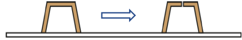
Figure 3: Study of the closed section longitudinal stiffener as two open section stiffeners
